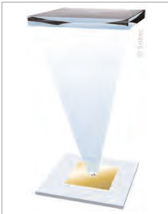
Figure 3. Schematic diagram of SOITEC's concentrated photovoltaic module.
