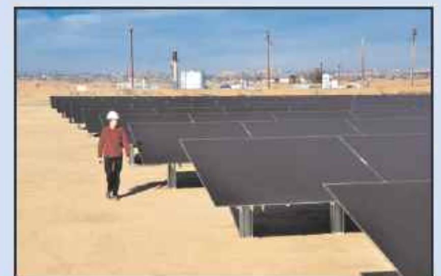
p67 Chevron's three-year Project Brightfield is to compare seven PV technologies, including Sharp, CdTe firm Abound, CIS firm Solar Frontier, and CIGS firms MiaSolé and Solibro.
