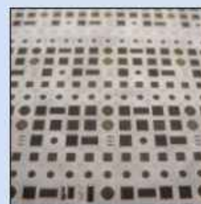
Cover: Photo of a solar cell wafer with different concentrator solar cell structures. Germany's Fraunhofer ISE has used theoretical calculations to optimize the front-side contacts and raise its European efficiency record for triple-junction III-V solar cells from 37.6% to 39.7%. p63
