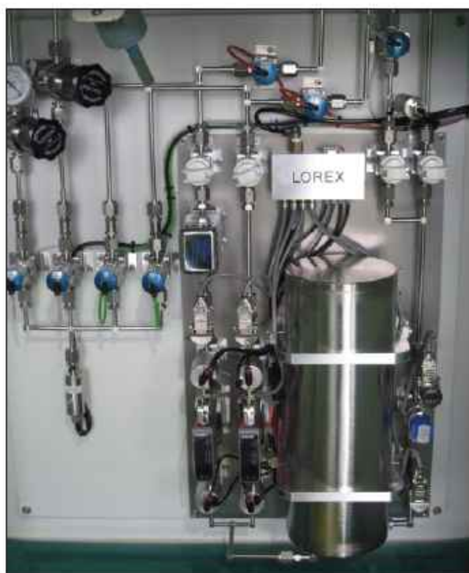
Piezocon Dopant Mixing System integrated in a valve manifold box.
