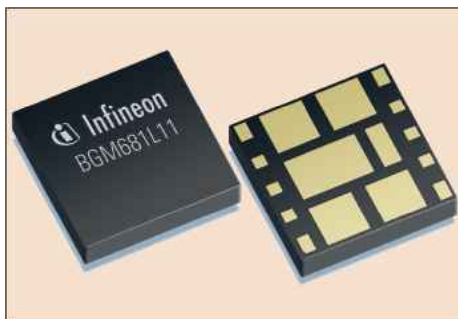
Leadless 2.5mm x 2.5mm x 0.6mm package of the BGM681L11 module.
