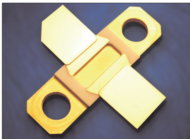
Laminate package for high-power GaN device.
