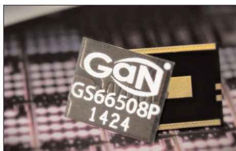
GaN Systems' GS6650P transistor used in winning design for Google Little Box Challenge.
