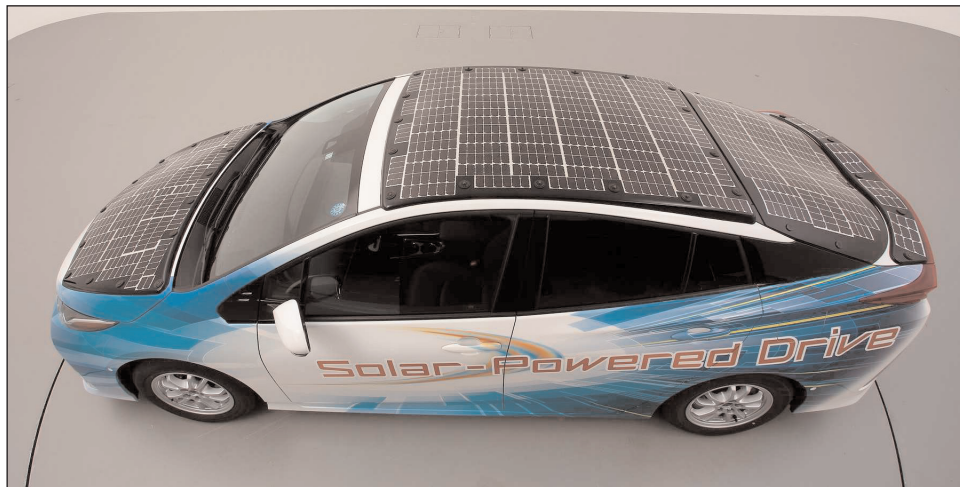
Toyota's Prius PHV solar demonstration car.
