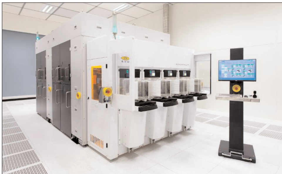
BONDSSCALE automated production fusion bonding system.
