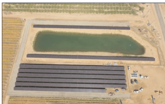
Solar Frontier's CIS modules installed in the Ag-solar installation in Delano, California. (Photo courtesy of Staten Solar.)
