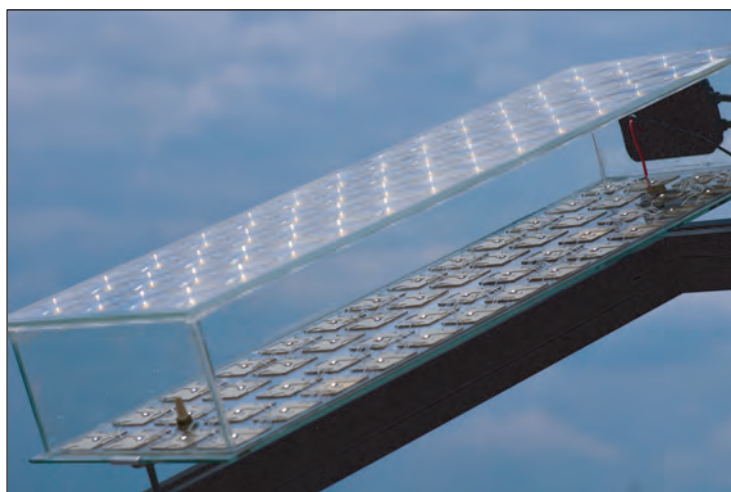
Fraunhofer ISE's latest, 36.7%-efficient FLATCON CPV module. ©Fraunhofer ISE/Photo: Alexander Wekkeli
