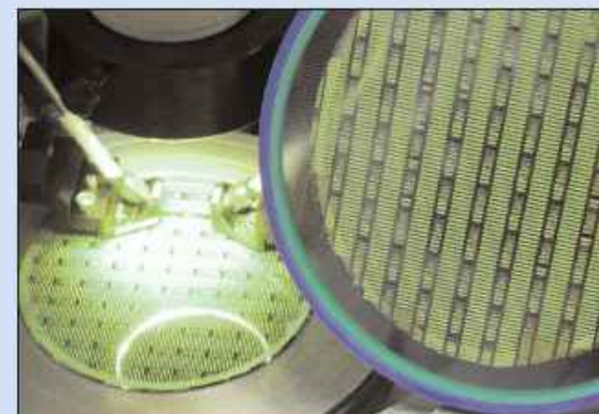
p8 Wafer fabricated using Nitronex's 48V GaN-on-silicon platform for wireless infrastructure.
