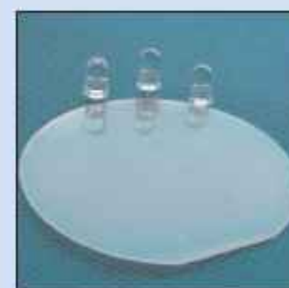
Cover: A 2" ZnO wafer made by Cermet, together with packaged LEDs. Cermet has licensed GaN-on-ZnO device technology, developed with the Georgia Institute of Technology, which enables the fabrication of LEDs that emit white light without the need for wave-length conversion by a phosphor. p16
