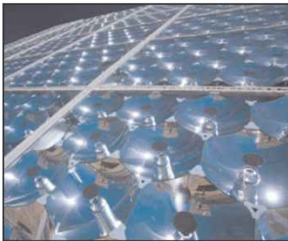
Close up of reflectors in SolFocus' CPV system.
