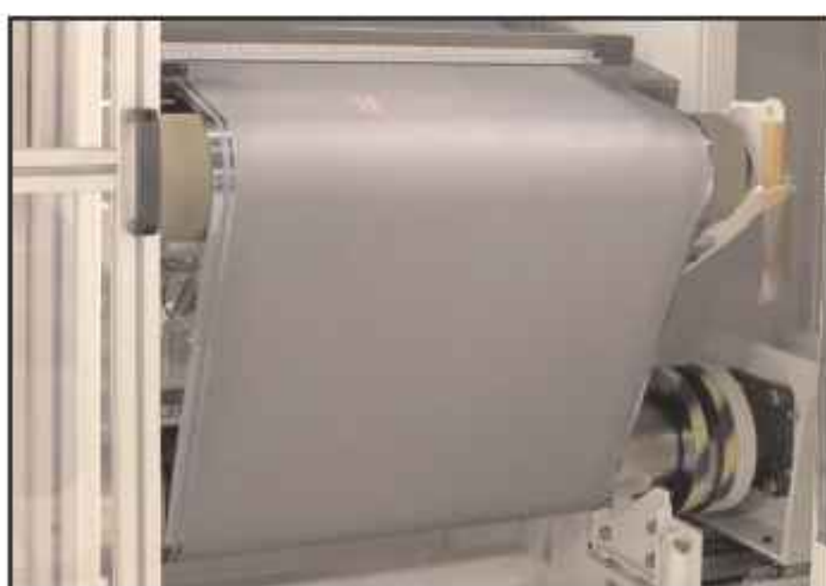
One roll of CIGS foil from Nanosolar's San Jose plant can deliver total power of 100kW.
