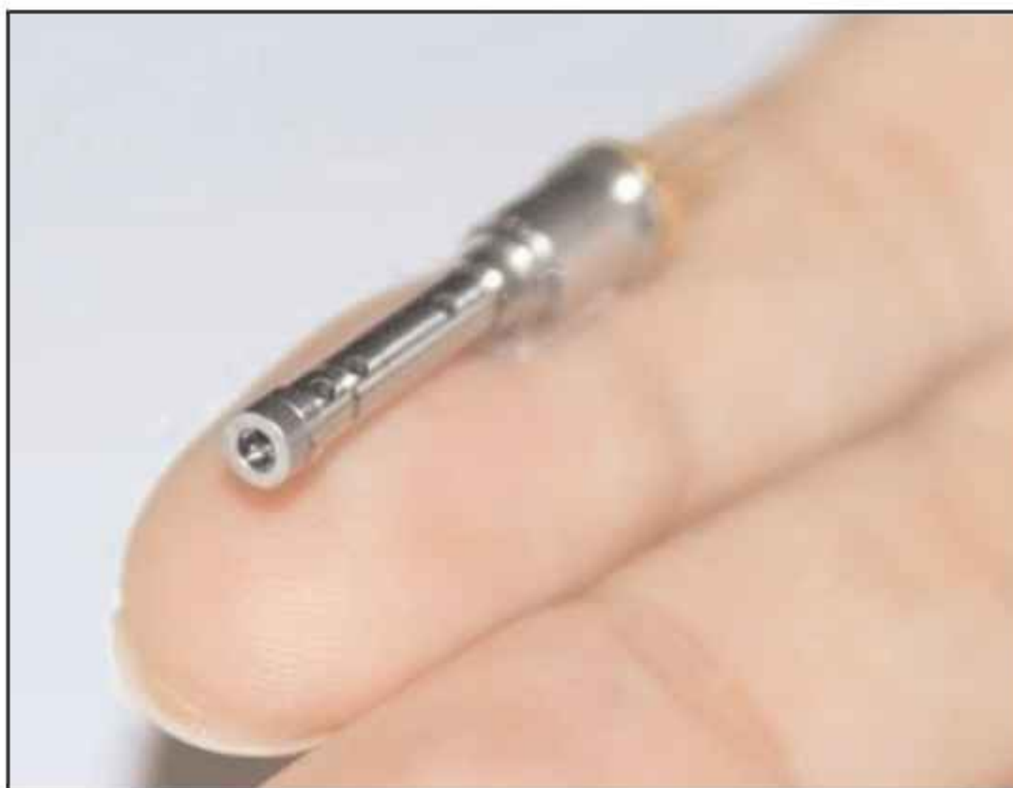
Figure 1. The 5.6mm-diameter quantum dot green laser. Because the quantum dot green laser can operate at 2V DC at temperatures up to 60°C without cooling and can be packaged in a 5.6mm-diameter TO-56 can (a generic package for laser diodes), QD Laser says that it meets the optimal power consumption and dimension requirements for
