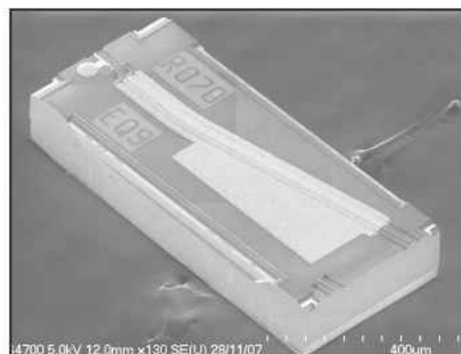
Monolithic chip inside CIP's R-SOA-EAM-1550.
