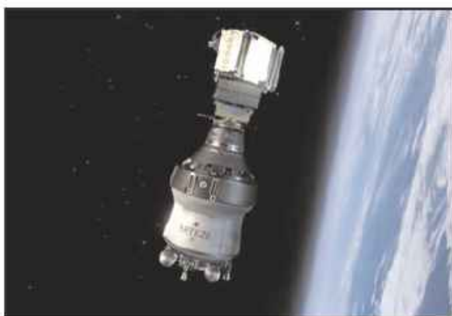
Artist's impression of SMOS atop the upper stage of Breeze launch vehicle.
