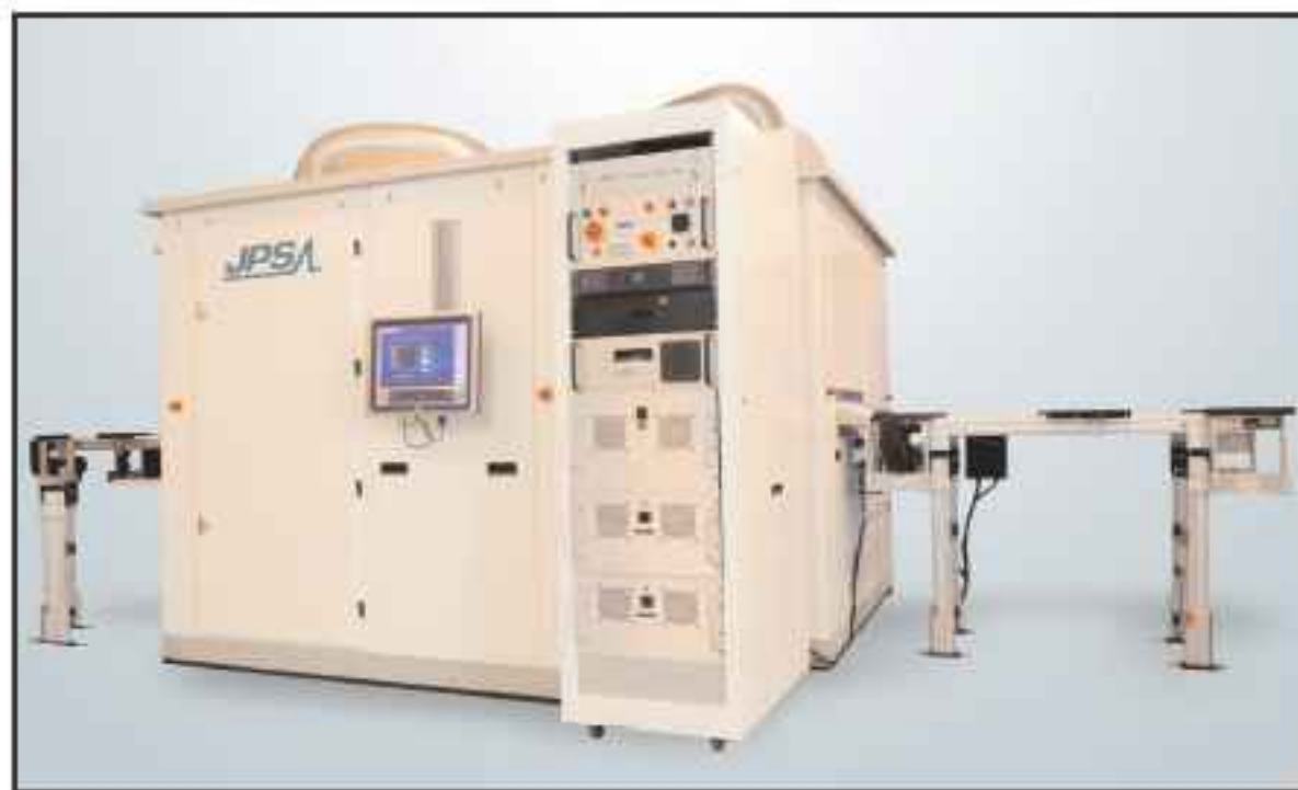
JPSA's PV-5000 thin-film photovoltaic laser scribing system.
