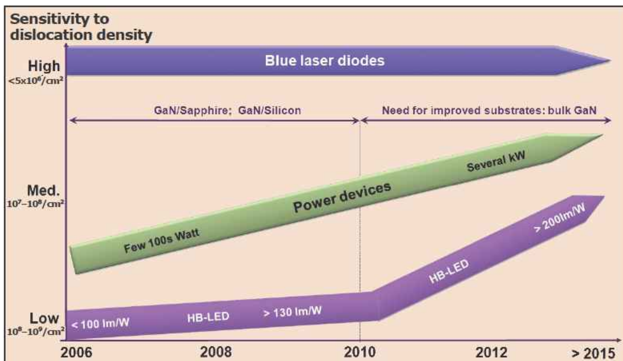
Sensitivity to dislocation density in active layer for various nitride devices.
