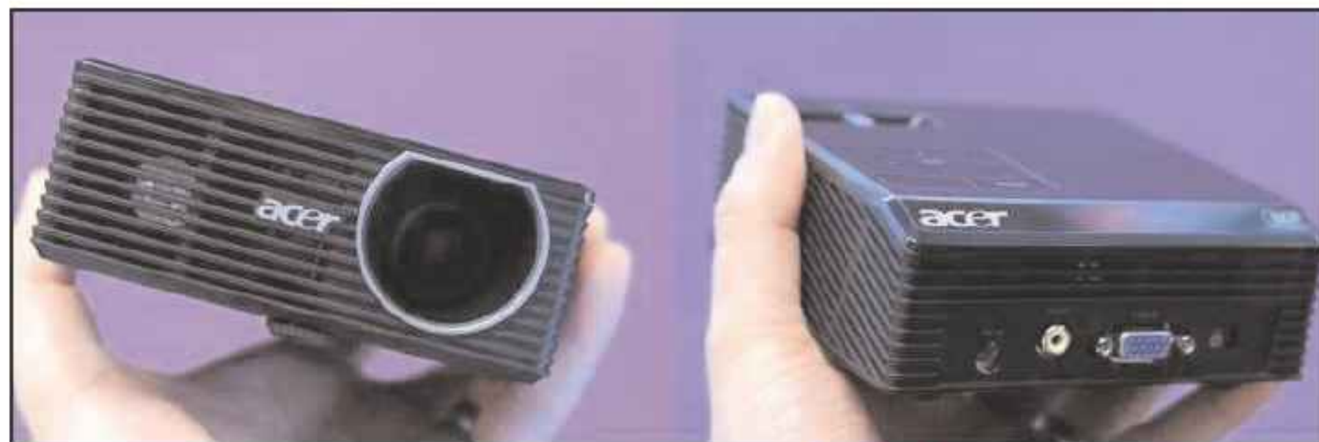
Acer's K10 pocket projector, incorporating a PhlatLight PT-39 chipset.
