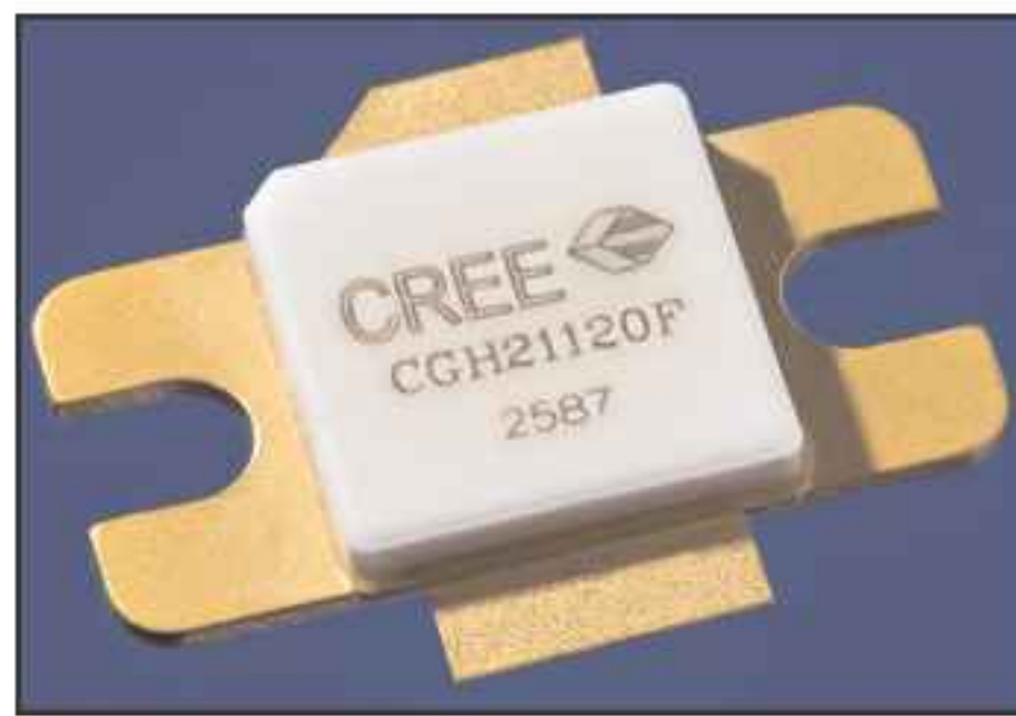
Cree's 120W CGH21120F GaN HEMT for the 1800–2300MHz range.
