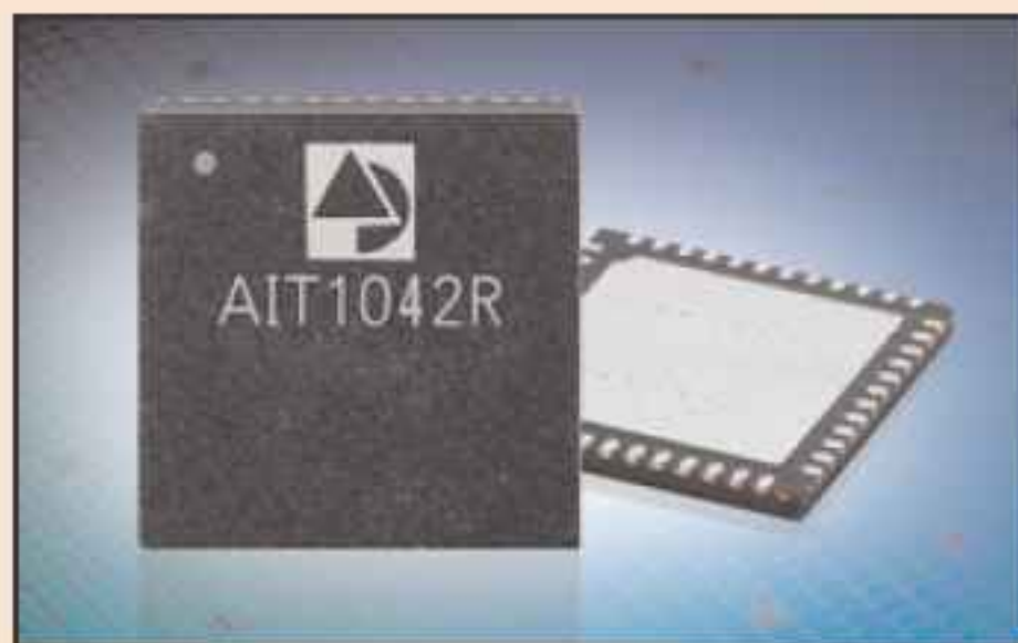
The AIT1042 integrated RF tuner.
