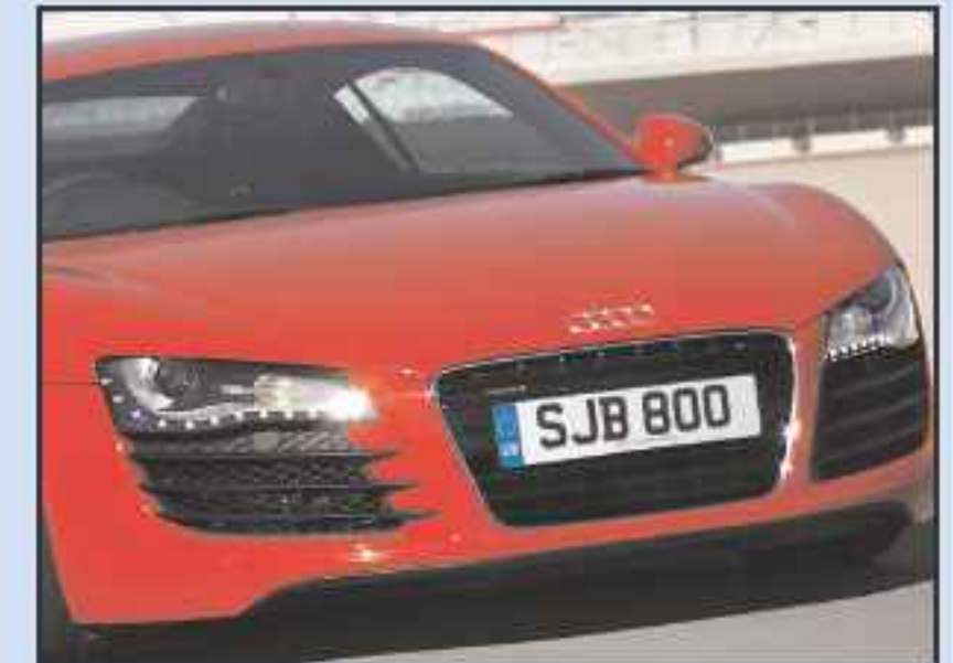
p43 New V10 version of Audi's R8, the first car with all-LED headlamps as standard.
