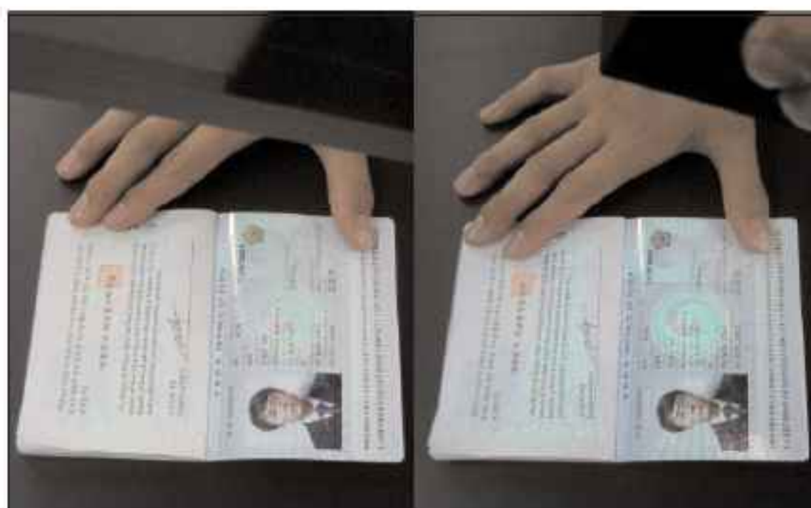
Comparison of fluorescent detecting function between existing UV mercury fluorescent lamp (left) and UV LED lamp (right).
