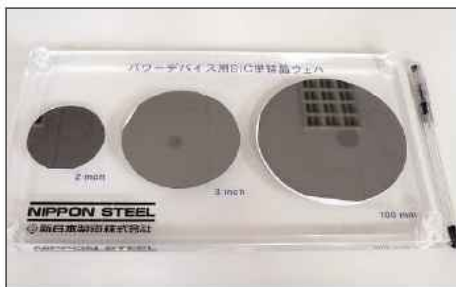
Nippon Steel's 2-4 inch (50-100mm) silicon carbide wafers.
