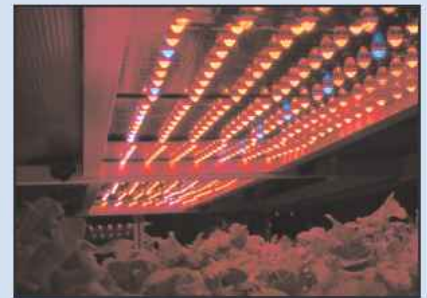
p38 Red and blue LEDs from Seoul Semiconductor used as an artificial light source to boost growth of plants.
