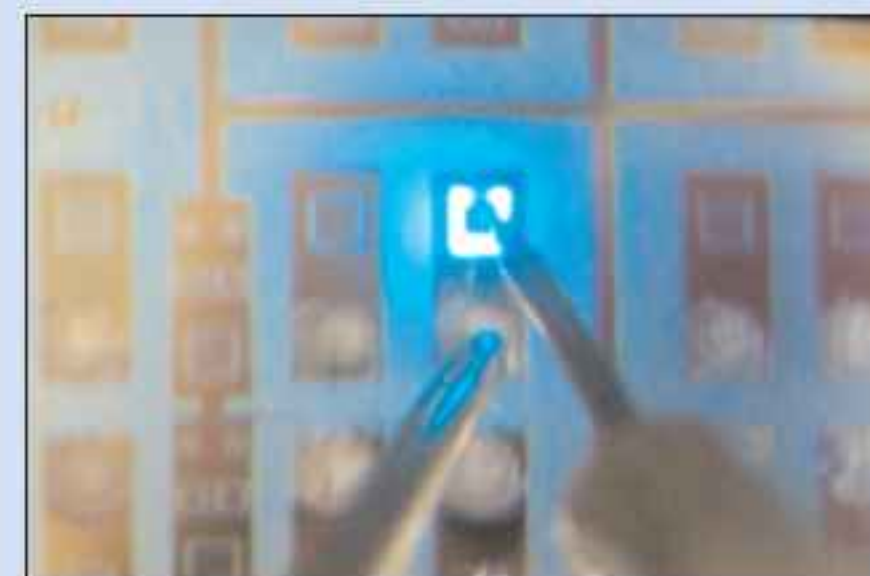
p27 Photograph of the first epitaxial structures for blue InGaN-based LEDs grown by hydride vapor phase epitaxy (courtesy of TDI).
