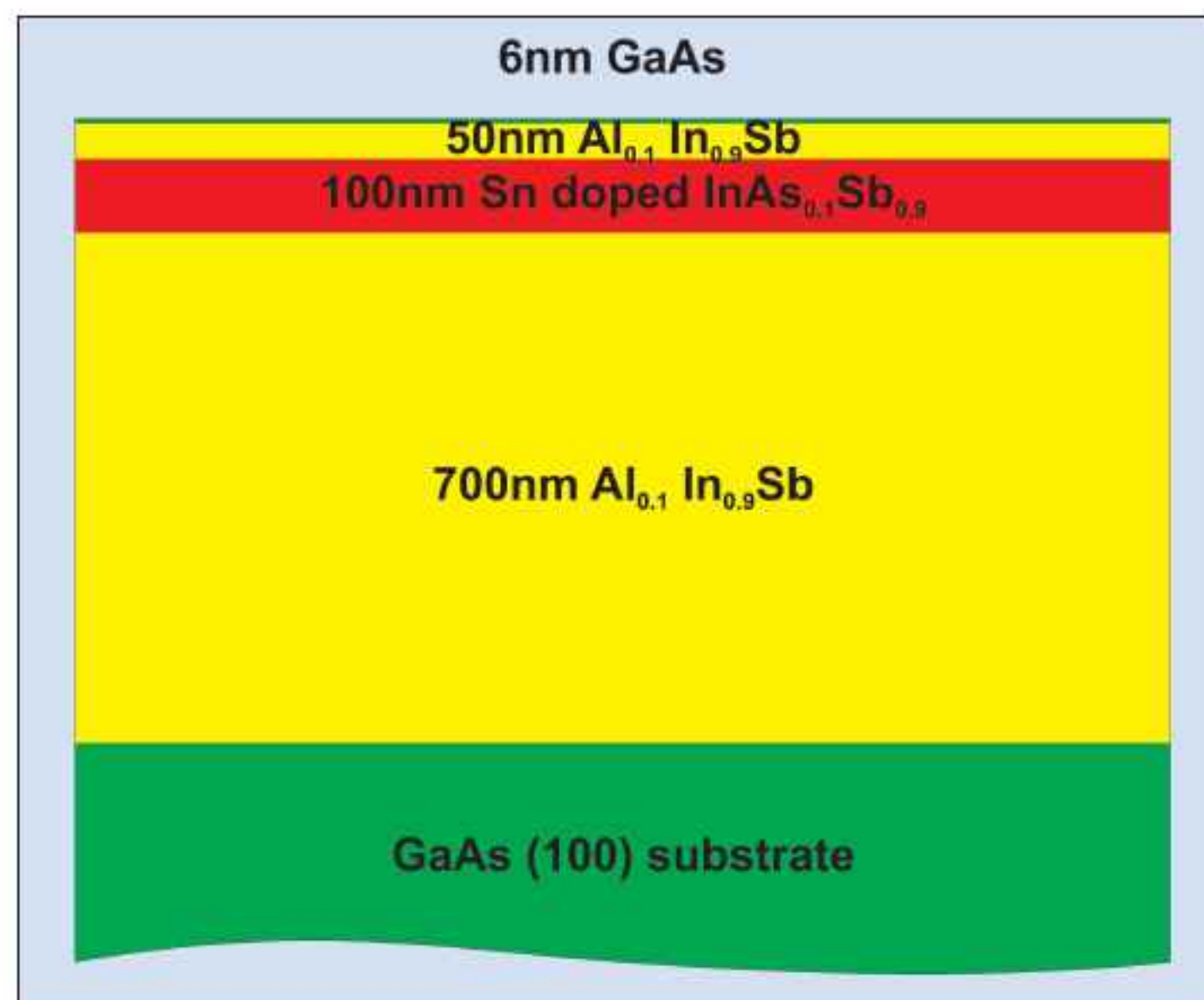
Figure 3. Schematic of Asahi Kasei's tin-doped antimony-based Hall sensor with improved mobility and temperature dependence.
