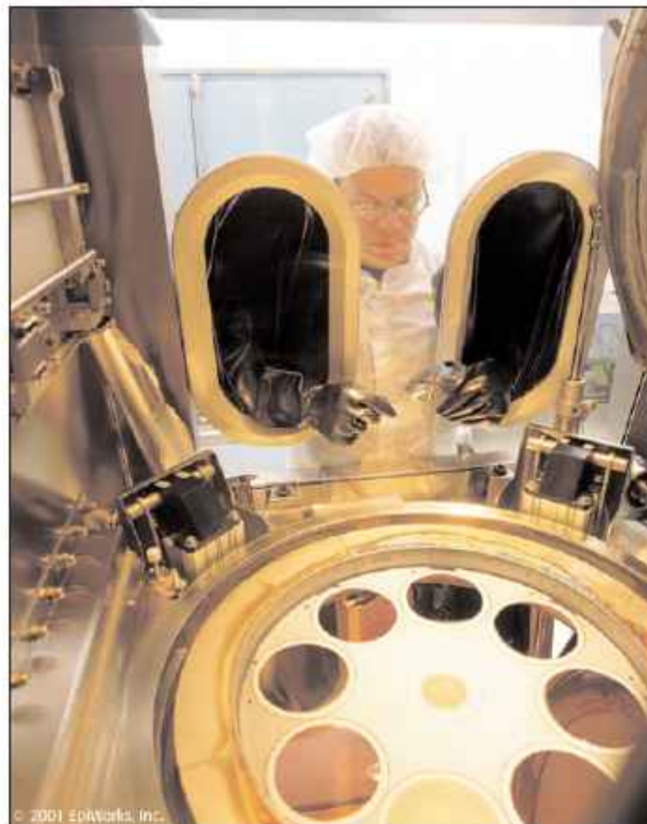
Aixtron 2600 MOCVD system identical to that installed in EpiWorks' recently completed Phase I expansion.
