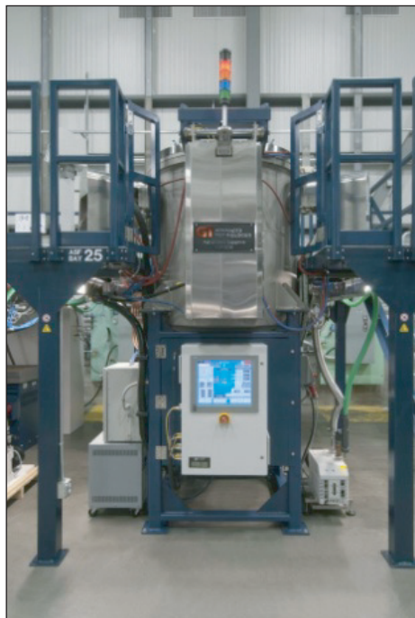
GT's ASF sapphire growth furnace uses the heat exchanger method (HEM) for producing boules and cores suitable for the LED industry.
