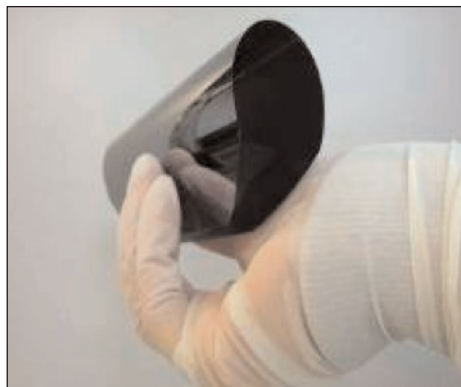
A free-standing 20 \mu m-thick silicon wafer, showing its flexibility.
