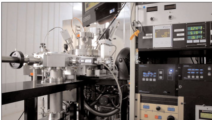
Reactir for Meaglow's CVD-based migration-enhanced afterglow deposition process.
