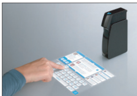
Light Touch from Light Blue Optics projects bright, high-quality video images in WVGA resolution using Opnext laser diode technology.
