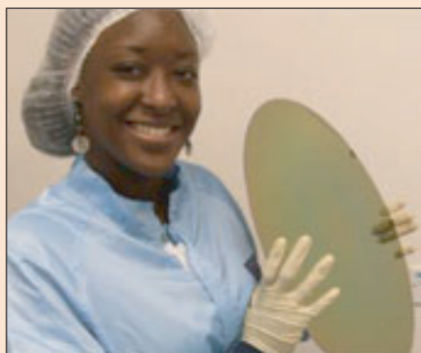
The first 450mm silicon wafer coated with PECVD SiO 2 .
