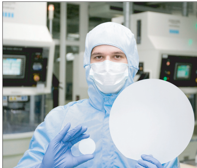
Monocrystal's 10" c-plane epi-ready sapphire substrate.
