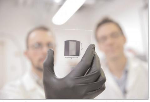
The UW–Madison engineers use a solution process to deposit aligned arrays of carbon nanotubes onto 1 inch by 1 inch substrates. The scalable and rapid deposition process was used to coat the entire surface of this substrate with aligned carbon nanotubes in less than 5 minutes.
