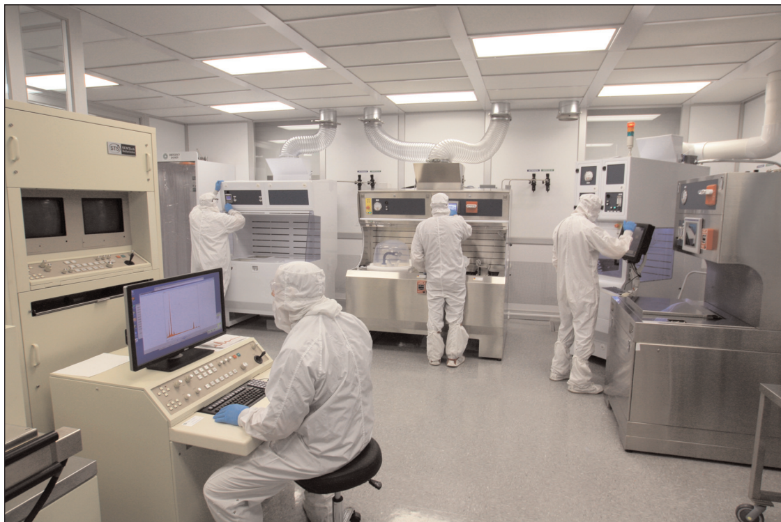
JST Manufacturing has an on-site applications laboratory where end-users can develop their process with various chemistries and conduct tests on real equipment ranging from immersion and spray tools to dryers.
